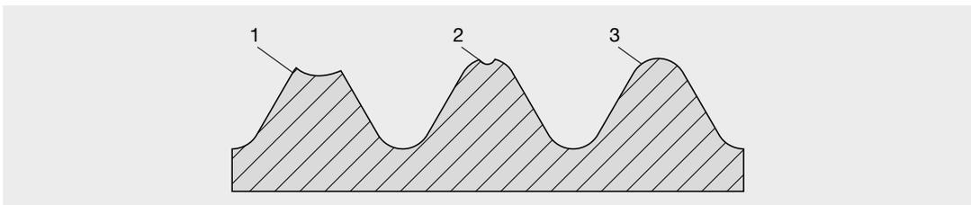
Figure 12: Degree of forming at the profile tooth
