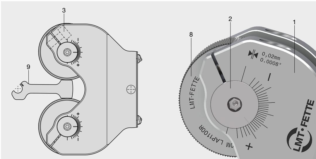
Figure 11: Adjusting the axle distance to workpiece dimension
