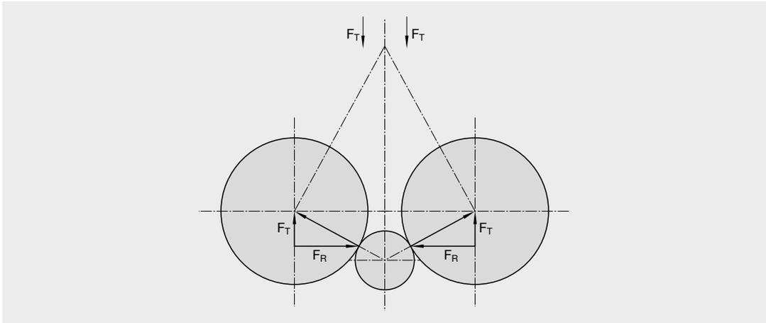
Figure 19: Forces occurring during the tangential rolling process
